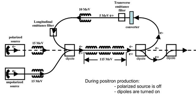
Figure 3: Schematics of CEBAF injector based positron generator/injector
