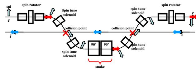
Figure 4: Spin rotation and stabilization in e-ring: spin injected to be vertical in arcs (using Wien filter); spin rotators matched with the cross bends of IPs. 180° solenoids are introduced between IP to inverse vertical spin between arcs of the twisted ring. Spin stabilizing solenoids introduced in sections with longitudinal polarization around detectors.
