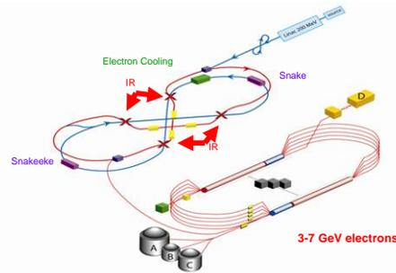
Figure 1: ELIC general layout. The e-collider ring (arcs) is also used as a large booster for the ion beam (before accumulating the e-beam).
