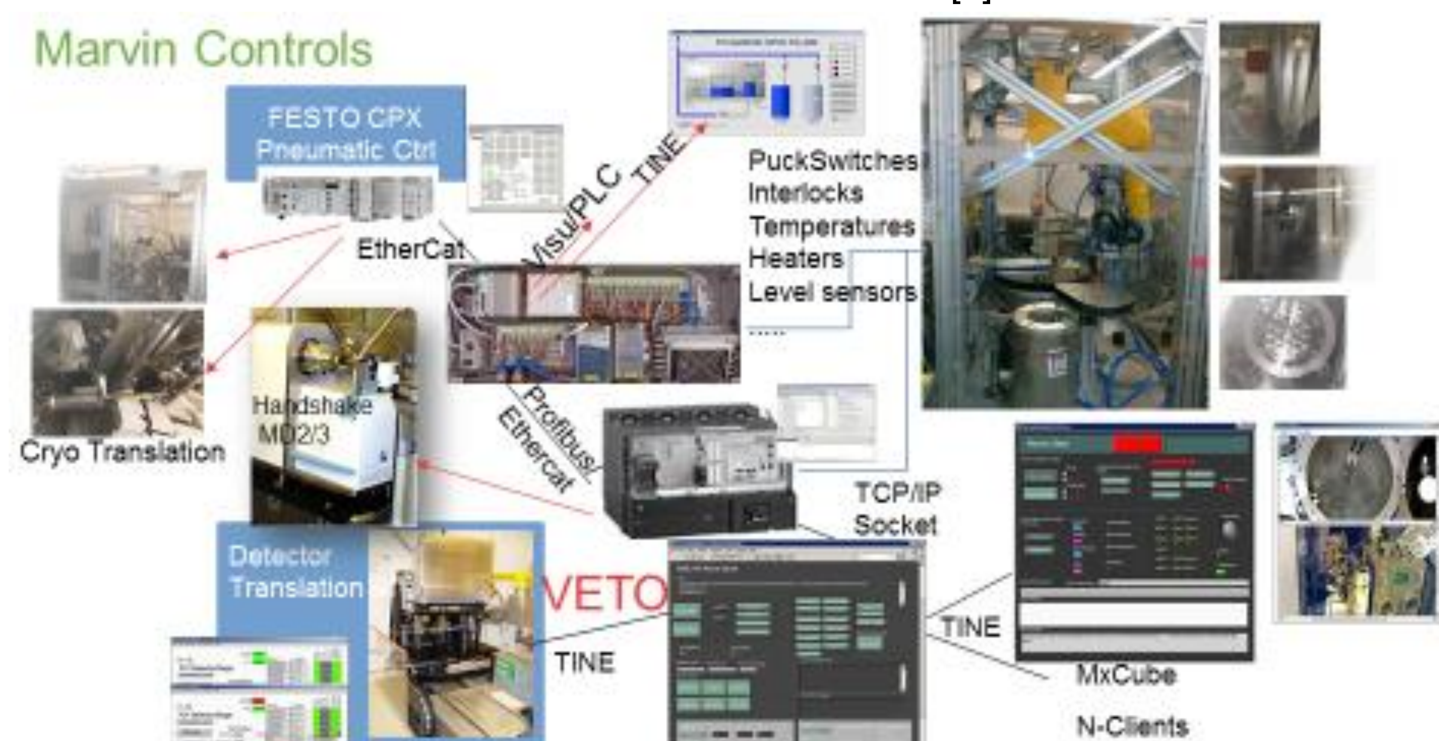
Figure 2. A sketch of the Controls involved in the Marvin Operation. Shown are the devices to be controlled and the Software controlling the devices
