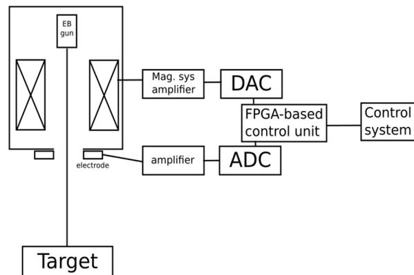
Figure 1: Scheme of the joint searing system.
