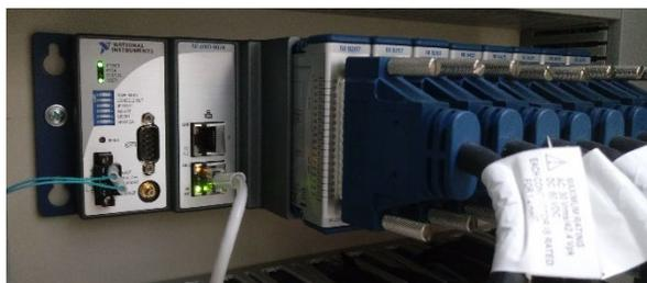
Figure 4: A model of the C-RIO controller with modules.
