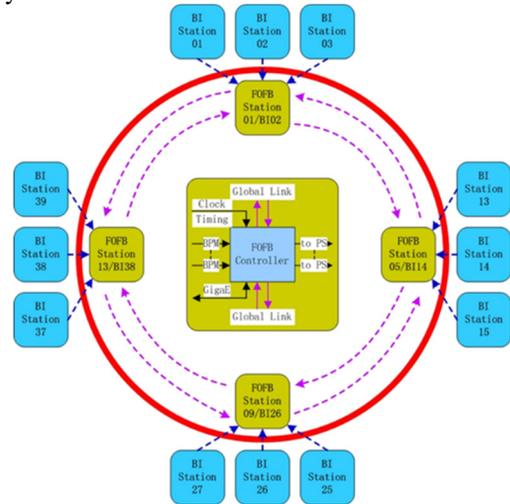
Figure 2: HEPS fast orbit feedback system architecture.
