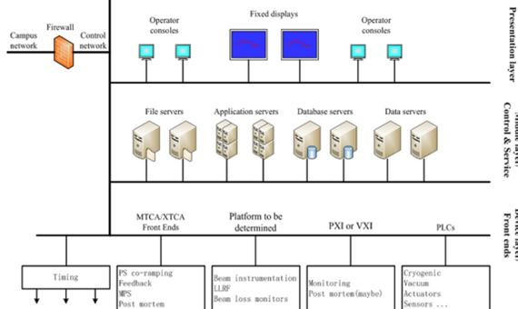
Figure 1: HEPS accelerator control system architecture.
