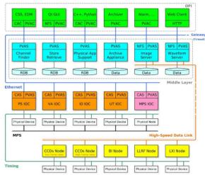
Figure 1: Architecture of the control system.
