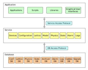
Figure 2: Architecture of the high level application.
