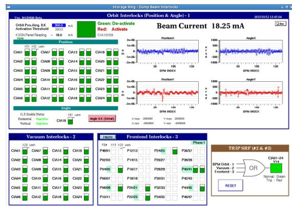
Figure 4: The machine protection system control page.
