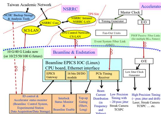
Figure 5: Accelerator control system interface with beamlines.
