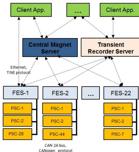
Figure 1: Magnet Control System structure overview.
