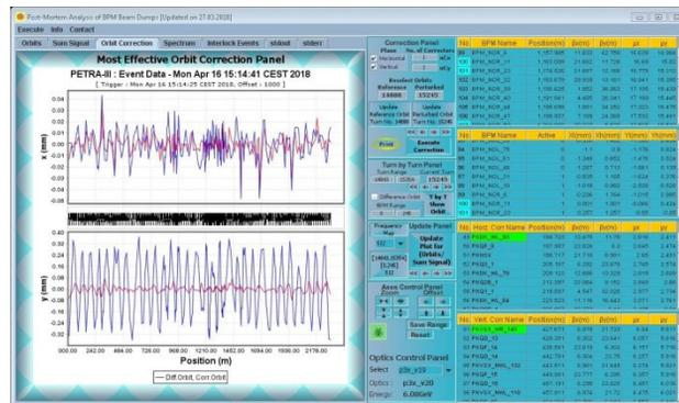
Figure 4: Vertical orbit correction for the Interlock Event on Monday 16 April 2018 at 15:14:41 which indicates that PKVSX\_WR\_140 vertical corrector as the source of orbit perturbation.
