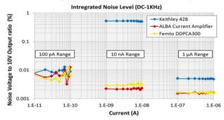
Figure 1: ALBA CA noise comparison with commercial electrometers.
