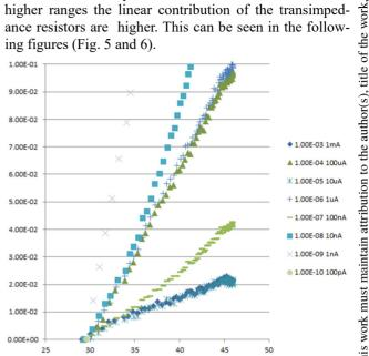
Figure 5: Offset current versus temperature, scaled to full scale.
