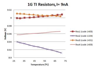
Figure 3: Study of temperature dependency of one of multiple resistors models analysed.
