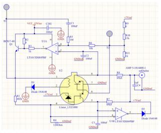
Figure 7: Schematic of voltage reference using the LTZ1000.
