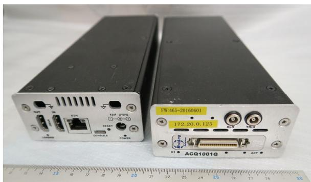
Figure 4: Outward of ACQ1001 with FMC module.
