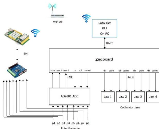
Figure 9: System block diagram of the updated system.
