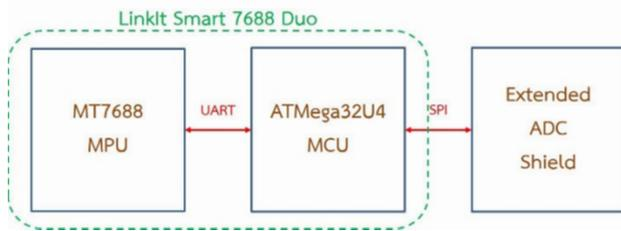
Figure 7: Interfaces between wireless development board and ADC.
