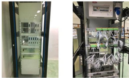
Figure 6: Equipment rack for PWM drive PCBs and DC power supply modules.
