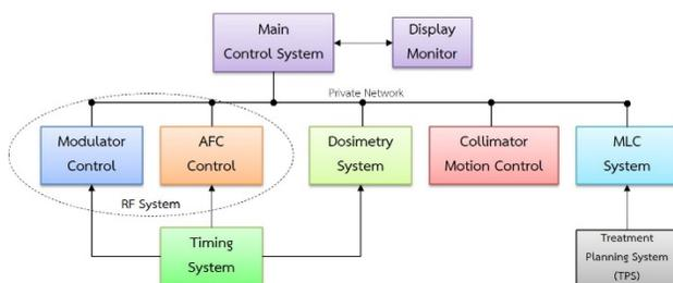
Figure 1: Network diagram of the machine prototype.
