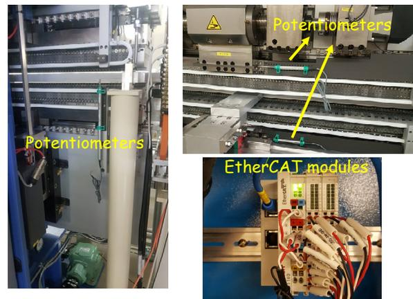
Figure 5: Potentiometers are installed to mirror the absolute encoders on the EPU48 and EPU46.
