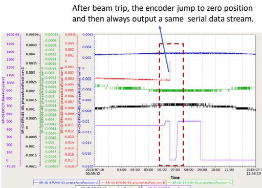
Figure 3: Case (3), the encoder stops sending a serial data stream.
