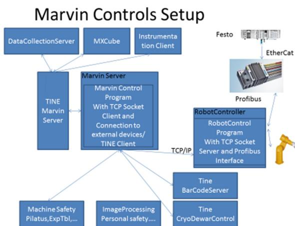
Figure 3: The MARVIN controls integrated in the beam-line controls.
