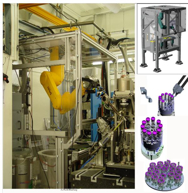
Figure 1: MARVIN mounting a sample on the MD3 Goniometer. And robot gripper, samples Pucks and Puck storage plate on the right.
