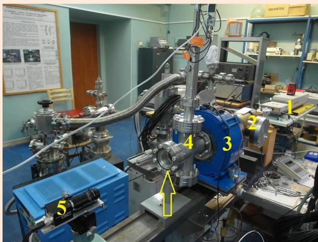
1 — LS-2134 laser, 2 — electron gun, 3 — focusing magnet, 4 — emittance measurement station, 5 — camera. The yellow arrow indicates the scintillating screen position.
