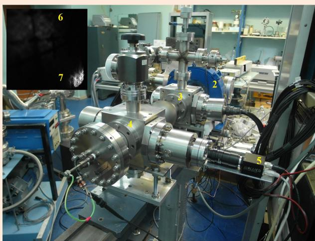
1 — LS-2134 laser, 2 — focusing magnet, 3 — wire profilometer, 4 — box with scintillating screen, 5 — camera, 6 — laser beam, 7 — electron beam
