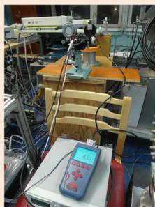
Main bench elements are 30-kV DC photogun with the transmissive photocathode, focusing magnet with correction windings, diagnostics equipment and a driver laser. Bench beamline vacuum is  $< 10^{-8}$  torr. A Faraday cup is used for electron bunch charge measurement. Laser pulse energy is measured by an Ophir Nova II power/energy meter equipped with PE25 pyroelectric sensor.
