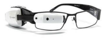
Figure 3: VUZIX M100 with gyroscope-based head tracking capability.
