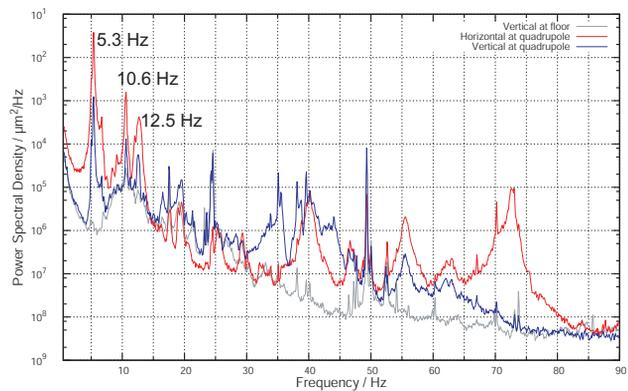
Figure 2: Magnet motion due to girder resonances.
