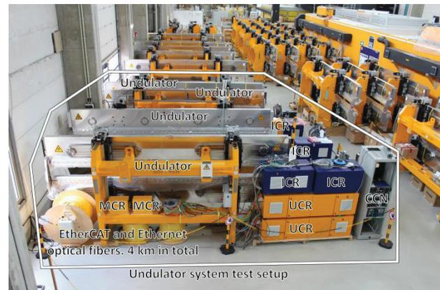
Figure 1: Undulator system test setup in the hall.
