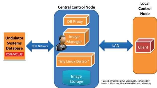
Figure 2: Schematic layout of the components of IDA.
