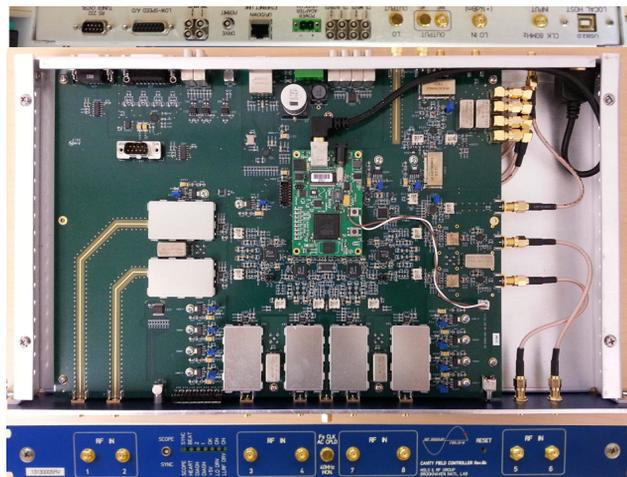
Figure 1: Picture of the CFC. The top and bottom of the picture shows the different IO on the back and front panels respectively.
