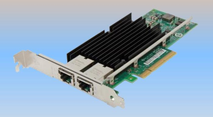
This Ethernet Converged Adapter X540-T2 is the latest 10GbE adapter with compatibility to 1GbE. Supports hardware IEEE1588, virtualization and Linux.
