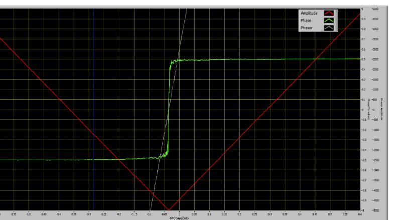
Open loop transfer curve of second harmonic modulator
