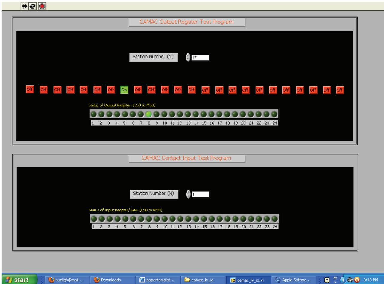
Figure 2: Snapshot of LabVIEW program testing CAMAC Output Register’s 8<sup>th</sup> channel (turning 8<sup>th</sup> channels relay ON/OFF) and also watching the status of all channels.
