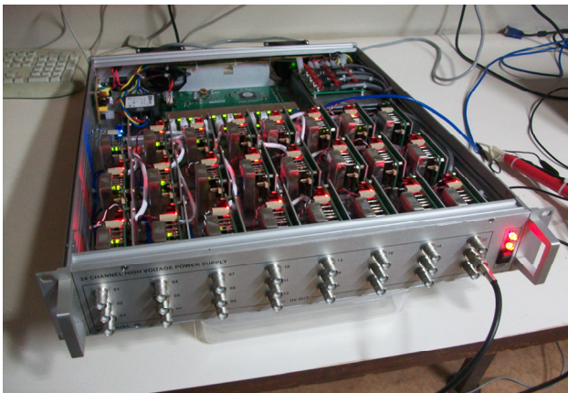
Figure 4: The inside view of a 24 channel unit.
