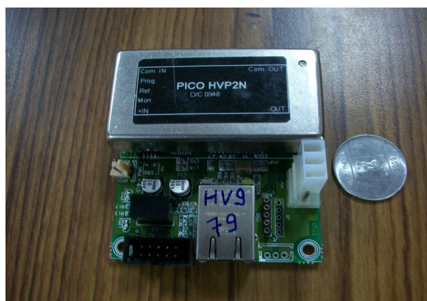
Figure 1: The single compact HV board with Ethernet.
