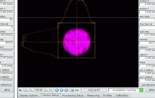
A GUI developed using Q-Tango supervises operation CCD of the The camera. graphical panel allows to deal with the CCD Tango device server (attributes API and commands) and visualizes the beam image at a selectable refresh rate and with the preferred false colour palette. It is possible to magnify the image, save a snapshot (TIFF) and store
