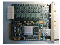
This picture shows the new µTCA ADC SIS8300 from the company Struck with the following features : • Ten 16-bit ADC 125MS/s sampling Two 16-bit DAC outputs Xilinx Virtex V FPGA
