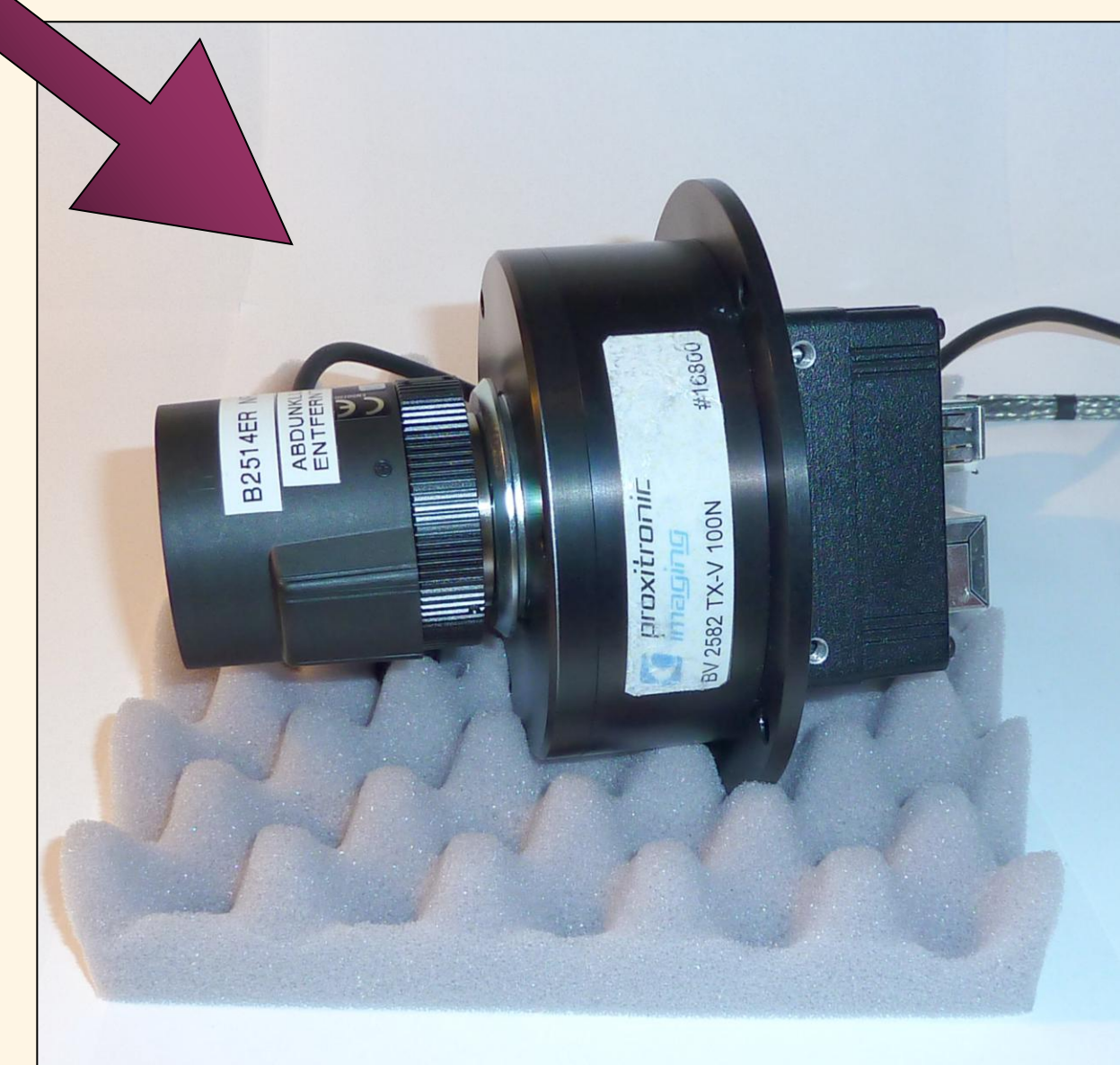
at the experiment: FireWire camera with image intensifier and iris
