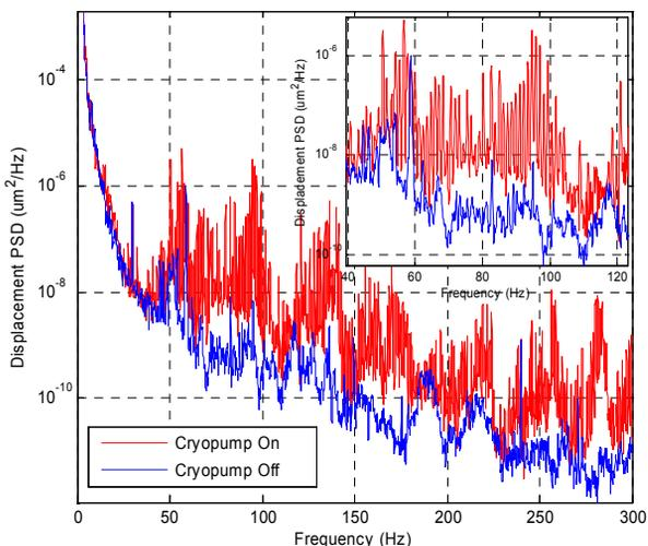
Figure 6: Cryopump induced vibration (in the vertical direction).
