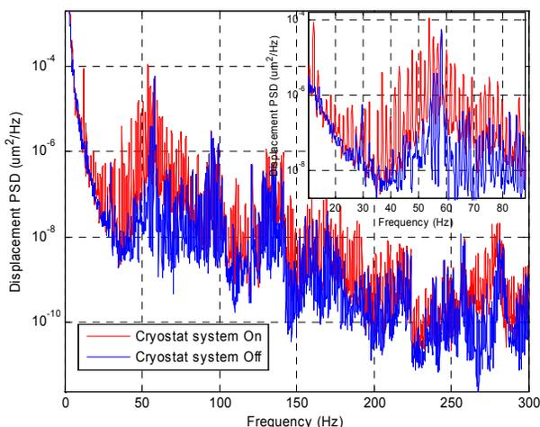
Figure 5: Cryostat system induced vibrations (in vertical direction).
