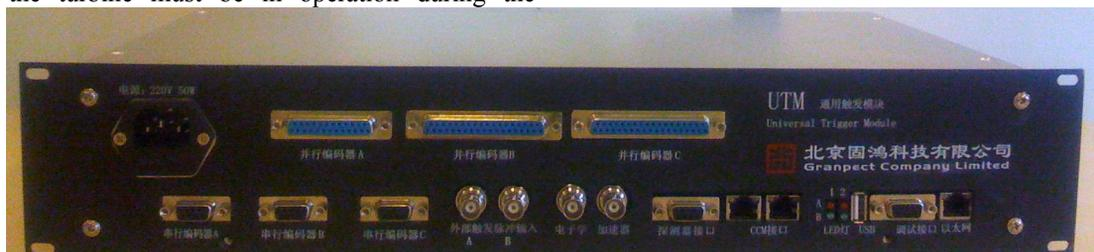
Figure 3: The front panel of the trigger module for industrial CT
