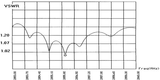
**Fig.5  $\rho \sim f$  curve of the BTW acc. tube**
