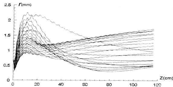
**Fig.4 BTW acc. tube radial beam envelope**
