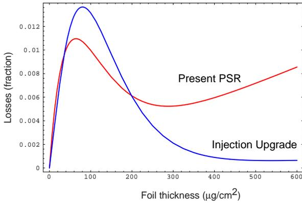
Figure 3. Total losses vs. foil thickness.
