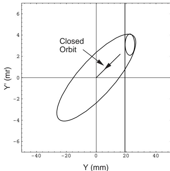
Figure 2. Closed orbit bump is collapsed linearly to zero during the injection period.
