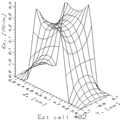
Figure 2: A typical MAFIA calculated 3-D field distribution in the accelerating gap.
