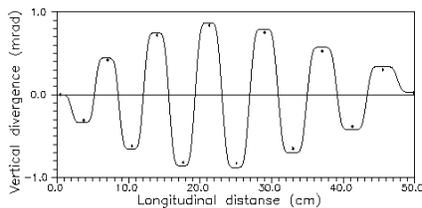
Figure 3: The overall accumulated dipole component effect in the IH structure.
