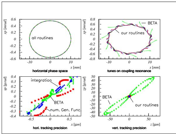
Figure 2: Comparison of tracking results for the original BETA routine and our Generating function and integration routines.
