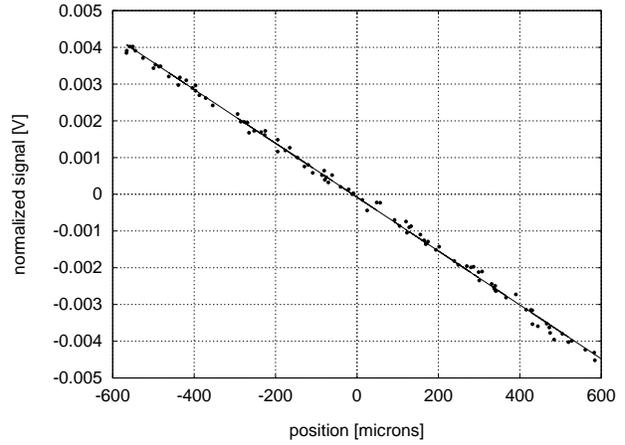
**Figure 6:** Linearized and signed amplitude of the dipole mode signal at station 2-2, frequency 4.139 GHz, as a function of the horizontal beam position determined with BPM's. The solid line is a linear fit.
