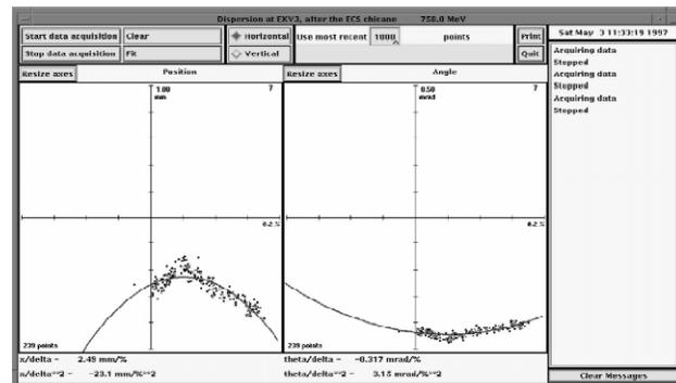
Fig. 4 Measured horizontal dispersions after the ECS chicane with the sextupole ESX1 set to  $+3.00 \text{ A}$
