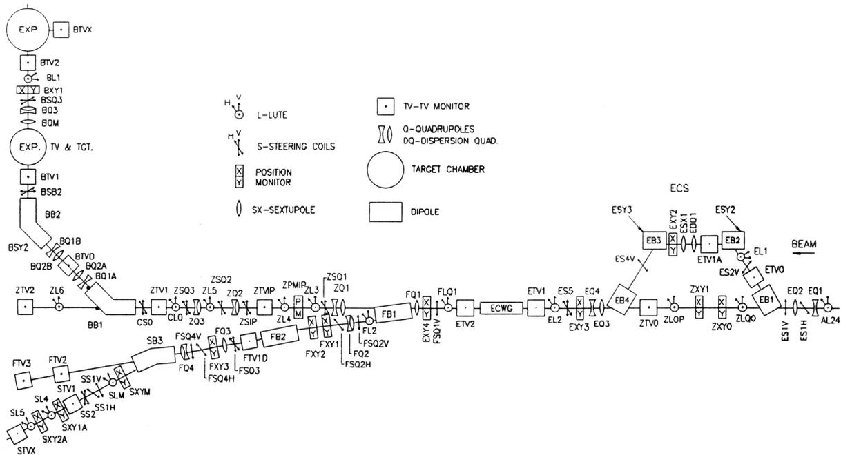
Fig. 1 Layout of the Bates beam switchyard showing the elements used to measure the dispersion
