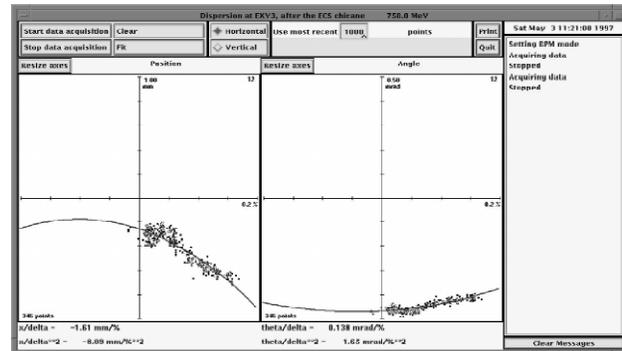
Fig. 3 Measured horizontal dispersion after the ECS chicane with the sextupole ESX1 set to  $+0.155\text{A}$
