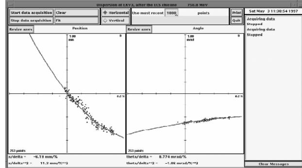
Fig. 2 Measured horizontal dispersion after the ECS chicane with the sextupole ESX1 set to  $-3.00 \text{ A}$
