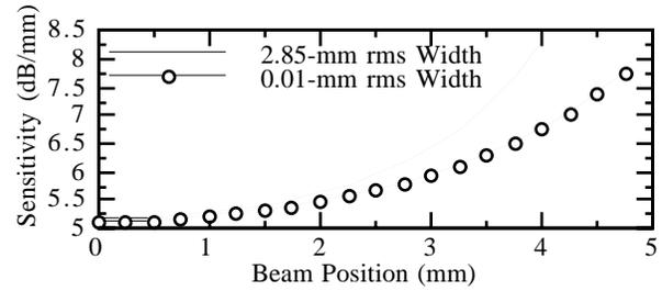
Figure 4. Diffuse- and thin-beam BPM sensitivity versus beam displacement from a BPM center. The BPM's radius and subtended angle were 7.0 mm and  $45^\circ$ , respectively.
