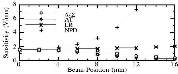
Figure 3. Combined sensitivities versus beam position for  $\Delta/\Sigma$ , AT, LR, and NPD processor transfer functions using a cylindrical 1.6-dB/mm-sensitive BPM.
