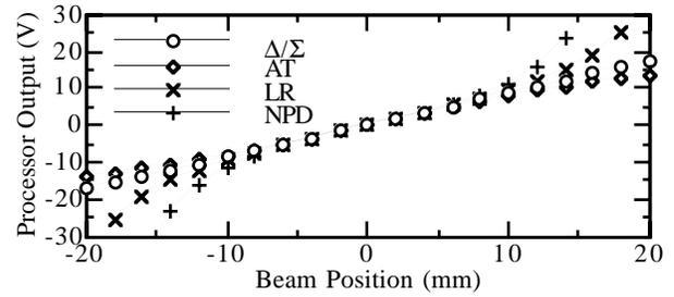
Figure 1. Processor output signal versus beam position for  $\Delta/\Sigma$ , AT, LR, and NPD transfer functions. A linear 0.87-dB/mm BPM response was used and all processors were normalized to have the same centered beam response.
