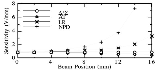
Figure 2. Combined sensitivities versus beam position for  $\Delta/\Sigma$ , AT, LR, and NPD processor transfer functions using a linear 0.87-dB/mm-sensitivity BPM.
