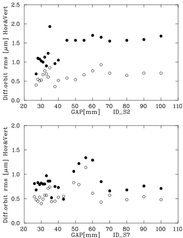
Figure 1. Residual change in orbit (rms) due to gap changes of ID#2 (upper) and ID#7 (lower) after correction coil calibration; solid circles - horizontal plane, open circles - vertical plane.
