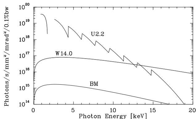
Figure 3. Performance of a mini-gap undulator in ELETTRA (2 GeV, 0.4 A,  $\epsilon_x = 7 \cdot 10^{-9}$  m rad,  $\kappa = 1$  %).
