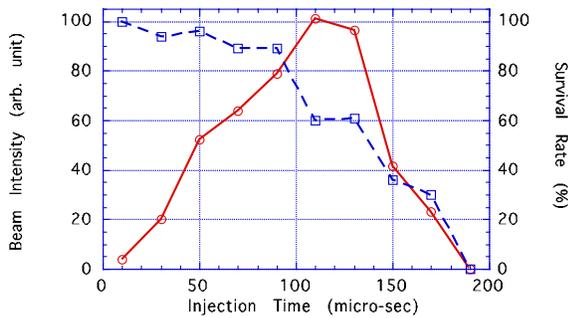
Fig. 1 A partial capture-efficiency just after the rf-capture and the survival rate after 1s. The solid and broken line indicate partial efficiency (arbitrary unit) and the survival rate (%), respectively.
