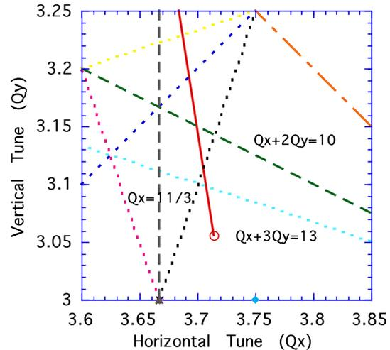
Fig. 2 The surveyed tune-line is indicated by the solid line. The dashed, broken and dotted line are 2nd, 3rd and 4th resonance line, respectively.
