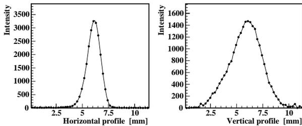
Figure 2: Horizontal and vertical profiles for optimum alignment, Pb ions, 270 GeV/c per charge
