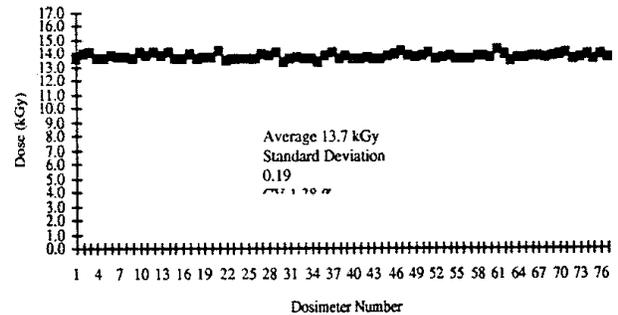
**Fig. 7.** Horizontal surface dose profile at the carrier midline.
