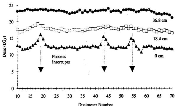
**Fig. 8.** Effect of a series of three process interruptions at various product depths at a conveyor speed of 1.2 meters per minute.
