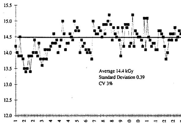
**Fig. 10.** Dose results from twelve process runs performed over a 20 day period measured at the reference monitoring position on the product box.
