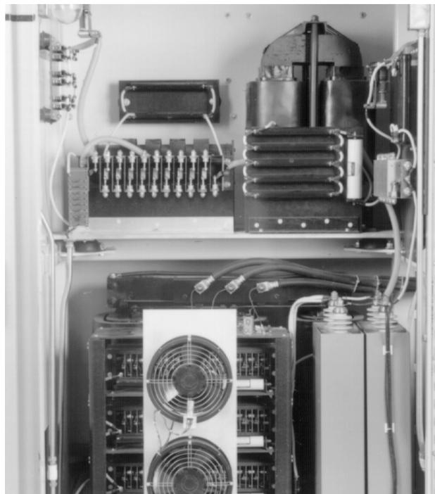
Fig. 4. Modulator High Voltage Power Supply
