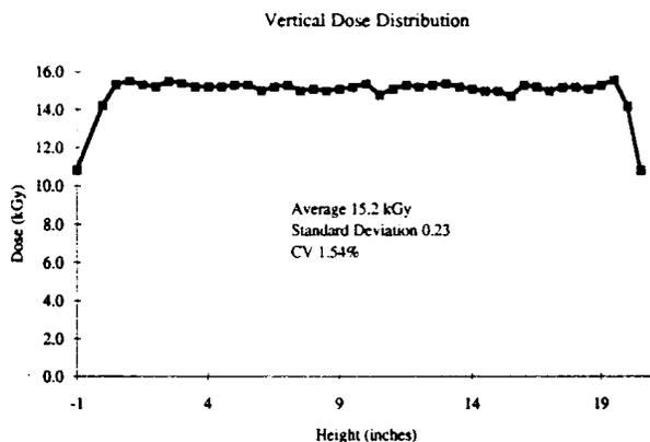
Fig. 2. Vertical dose distribution (scan width) at the surface of a 0.1 g/cc uniform density foam phantom.
