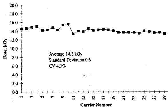
**Fig. 9.** Results of thirty carrier measurement on a single process run measured at the reference monitoring position on the product box.
