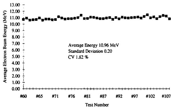
**Fig. 11.** Plot of 47 energy determinations from penetration range measurements in aluminum block over an eight month period.
