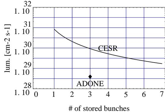
Fig. 2 - Luminosity vs. number of stored bunches in CESR at 112 mA (continuous line). The luminosity achieved at ADONE for the FENICE experiment is shown for comparison.
