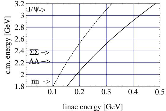
Figure: 1 Invariant mass vs. electron beam energy in head on collision with the stored positron beam of energy 5.3 GeV (continuous line) and 8 GeV (dashed line).
