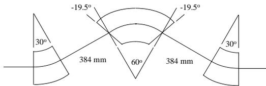
Figure 2. Boeing chicane composed of three  $n=1/2$  dipoles.
