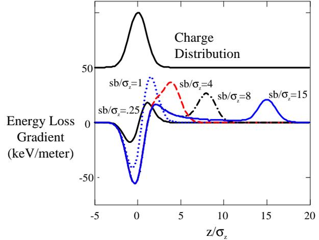
Figure 1. Evolution of the energy loss gradient along the microbunch for 1 nC and a bend radius of one meter. The CSR-induced gradient reaches equilibrium for  $sb/\sigma_z > 6$ . The transient radiation produced when the bunch enters the bend is seen propagating to the right for  $sb/\sigma_z > 4$ .
