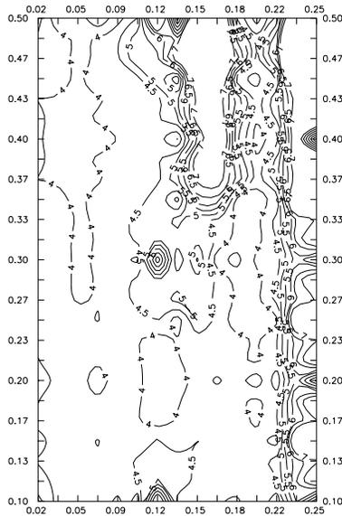
Figure 3: Contour plot of maximum betatron amplitude  $A_{max}/\sigma_0$  vs rms bunch length  $\sigma_s$  and tune  $\nu_y = \nu_x = \nu$ ,  $\xi = 0.05$ ,  $\Delta\vartheta = 0.002$ , 75,000 turns.
