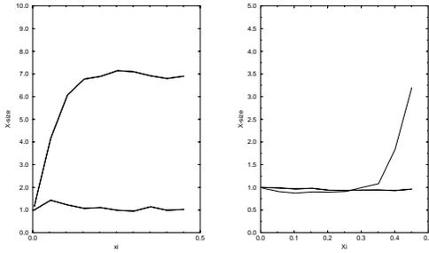
Figure 2: Beam size after 50,000 turns versus  $\xi$ . The upper curve corresponds to the short strong Gaussian bunch, the lower one — to the strong counter bunch with the ”inverse beta-function” distribution. The beta-function at IP is 25 cm. **a** – left figure – tunes are equal to  $\nu_x = \nu_y = -0.01$ ; **b** – right figure – tunes are equal to 0.05.
