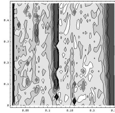
Figure 4: Contour plot of the maximum betatron amplitude vs. tune  $\nu$  (horizontal axis) and the tune difference between two IPs  $\Delta\nu_{1,2}$  (vertical axis) for the round beams.  $\Delta\vartheta = 0.002$ , 100,000 turns.
