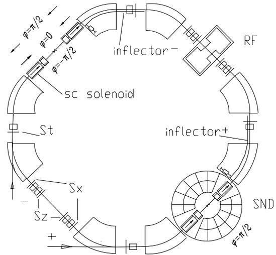
Figure 1: Layout of the VEPP-2M collider. Arrows inside solenoids indicate the direction of the longitudinal magnetic field.
