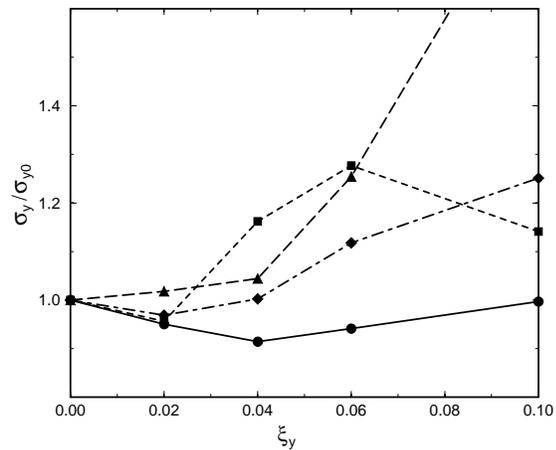
Figure 4: Equilibrium beam sizes for the different schemes: R (circles), M1 (squares), M3 (diamonds), and F (triangles). The decrease of the beam size for a small  $\xi$  occurs due to the dynamic beta effect.
