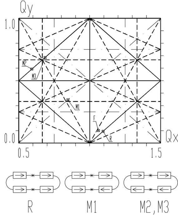
Figure 2: The grid of working resonances up to 4th order. Sextupole resonances are shown as bold dashed, betatron resonances of 4th order as long-dashed. For the Möbius cases  $Q_x$  and  $Q_y$  should be read as  $Q_+$  and  $Q_-$  for “+” and “-” modes. At the very bottom the schemes of solenoids polarities are shown for the described cases.
