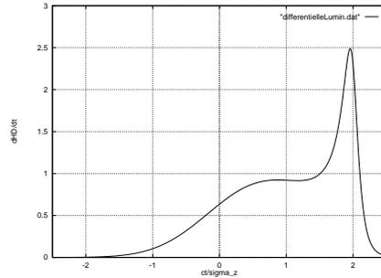
Figure 1: Differential luminosity  $\frac{1}{\mathcal{L}_0} \frac{d\mathcal{L}}{dt} = f(ct/\sigma_z)$  for  $D = 0.7$ .
