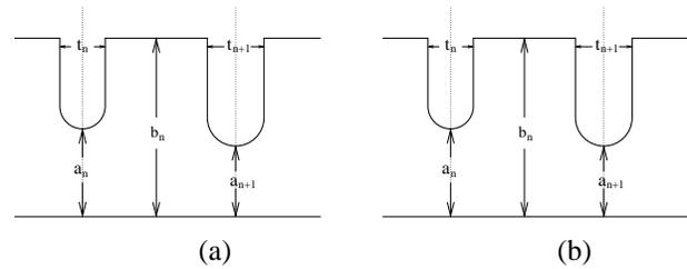
Figure 1: (a) The dimensions of a typical cell; (b) Variations of cell dimensions.
