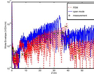
Figure 6: For JLC: Wake envelope comparison between FEM and open-mode method; the circles are measured data.
