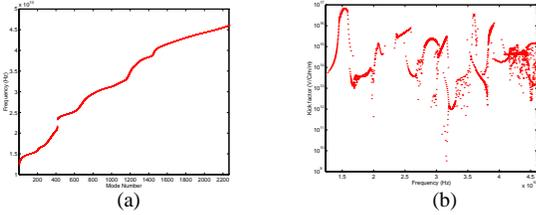
Figure 4: Dipole modes for NLC: (a) frequency vs mode number; (b) kickfactor vs frequency.
