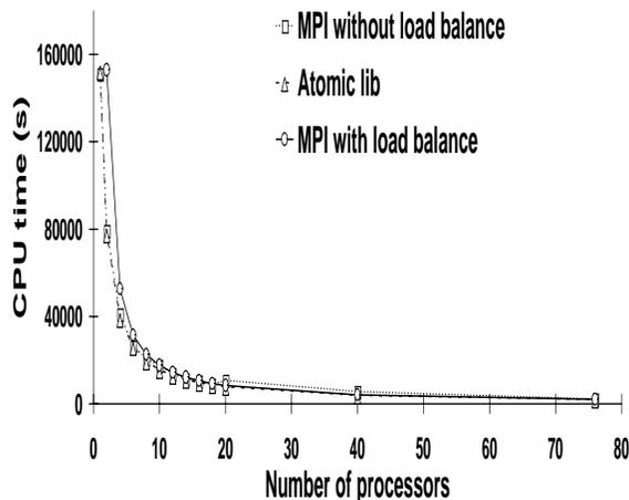
Figure 1: Performance of the first parallel algorithm. The total CPU-time is depicted as a function of  $N_{proc}$ .
