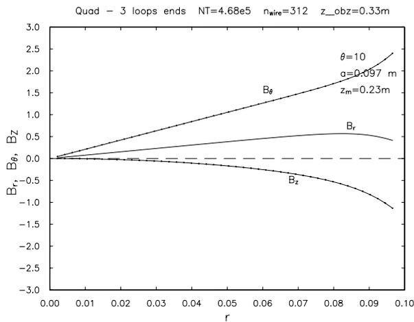
Figure 2: Magnetic Field of the Quadrupole along  $r$
