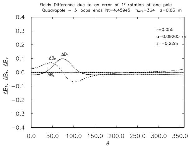
Figure 7: Field errors due to 1° shift in the center of one loop
