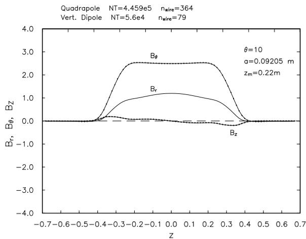
Figure 8: Combined Field of the above Quadrupole and Dipole at  $r = 0.055 m$ .
