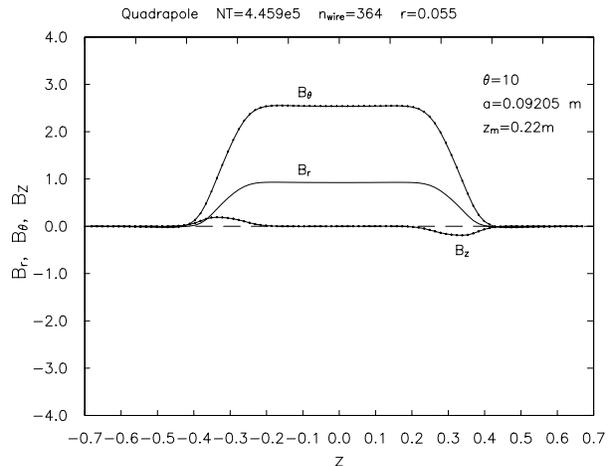
Figure 1: Magnetic Field of the TESLA Quadrupole for  $r < a$
