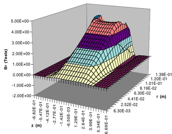
Figure 4: Magnetic Field  $B_r$  of the TESLA Quadrupole along  $z$  for  $0 < r < 1.5a$
