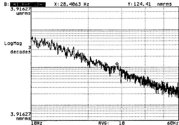
Figure 5: Damping from two Lead Bricks
