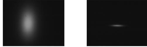
Figure 2: Beam images from dipole ADI01 4 degree exit port corresponding to E=120 MeV (left) and E=1.37 GeV (right).
