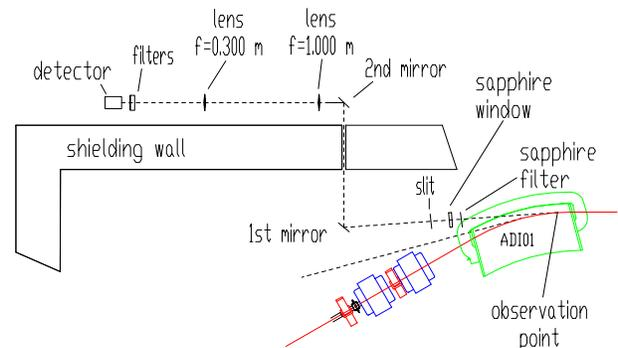
Figure 1: The LNLS UVX optical characterization bench.
