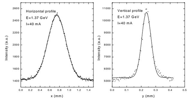
Figure 3: Horizontal (left) and vertical (right) beam profiles for E=1.37 GeV and I=40 mA. The solid curve is a gaussian fitted to the experimental data (dots).
