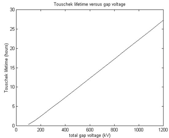
Figure 1. Calculated Touschek Lifetime vs. Gap Voltage
