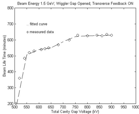
Figure 2. Lifetime vs. Gap Voltage ( Wiggler Gap Opened)
