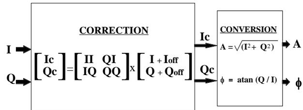
Figure 3. Software algorithm for the I/Q Demodulators
