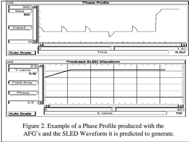
Figure 2. Example of a Phase Profile produced with the AFG's and the SLED Waveform it is predicted to generate.
